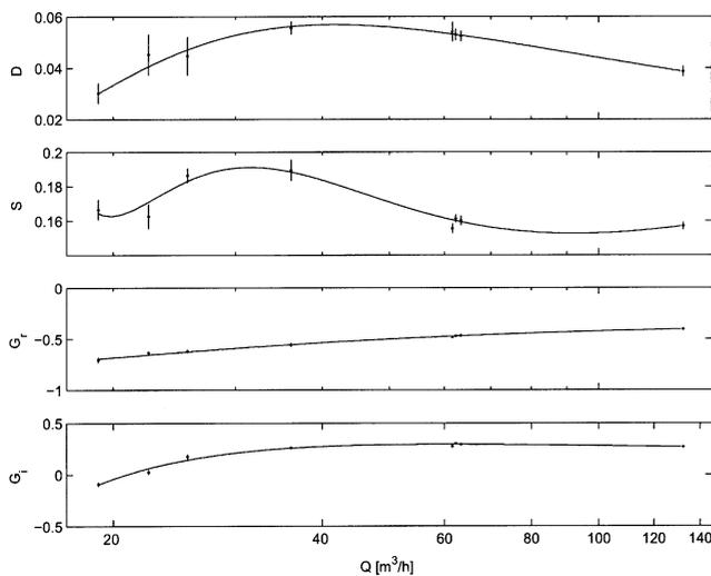
Fig. 1. The dependence of the features  $D$ ,  $S$ , and  $G = G_r + iG_i$ , defined in Section 3 for a correctly mounted flowmeter. The points correspond to measurements ( $1-\sigma$  errorbars), the curves to polynomial fits.
