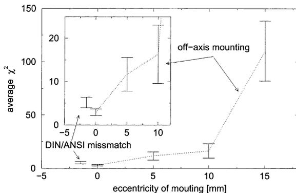
Fig. 3. Average values of  $\chi^2$  derived from the sensor signal in order to detect inappropriate mounting. The data point for DIN/ANSI mismatch was shifted to the left. The inset is a blowup of the low- $\chi^2$  region.
