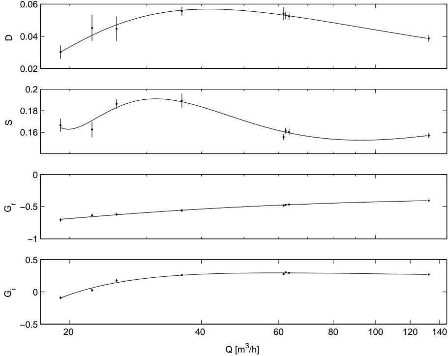
Figure 1: The dependence of the features  $D$ ,  $S$ , and  $G = G_r + iG_i$ , defined in Section 3 for a correctly mounted flowmeter. The points correspond to measurements ( $1\text{-}\sigma$  errorbars), the curves to polynomial fits.
