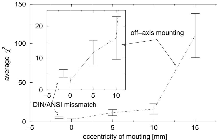
Figure 3: Average values of  $\chi^2$  derived from the sensor signal in order to detect inappropriate mounting. The data point for DIN/ANSI mismatch was shifted to the left. The inset is a blowup of the low- $\chi^2$  region.
